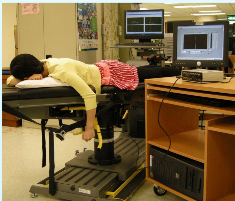
Fig 1. The HUMAC® / NORM™ Testing and Rehabilitation System for examination of ankle proprioception
